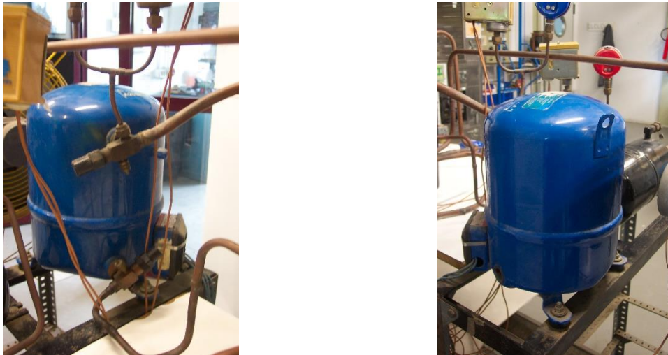
Figure 3. Hermetic compressor used in the Heat Pump studied
